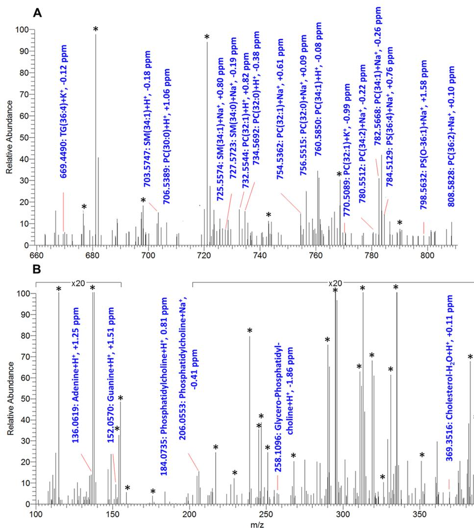
**Figure 2.** Mass spectrum acquired from a single 7  $\mu\text{m}$  pixel for mass range  $m/z = 620\text{--}810$  (A) and  $m/z = 100\text{--}380$ . (B) Identified compounds are labeled with measured mass, compound name, and mass deviation. See Table S-1 in the Supporting Information for more details. Background peaks (e.g., from matrix or sample support) are marked with an asterisk.
